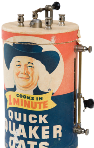
In the 1920s, radios weren’t cheap. Many families built their own, such as this reproduction . Wire was wound inside the oatmeal box; a sliding contact allowed for tuning. But you still needed earphones and antenna wire, Belanger says.
