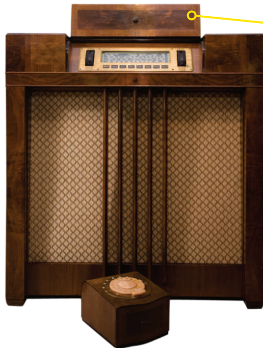
This 1939 Philco Radio Model 39-116 with “mystery control” was one of the first with a wireless remote, Belanger says. Using the phone-book-size remote control, listeners could select from eight stations they had programmed when they bought the radio.
