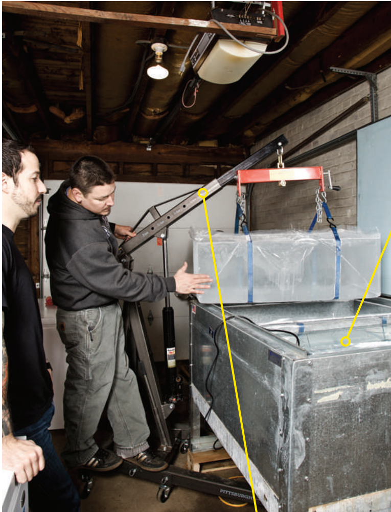
Marindin uses an engine hoist to lift ice out onto a prep table, but he doesn't cut it immediately. Otherwise, says Ambrose, left, cracks form inside the ice, making clear cubes impossible. The ice needs to temper (be brought slowly to a warmer temperature) for a few hours so it will be more pliable.
