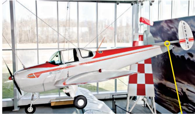
Made of mostly aluminum, the Ercoupe weighed about **845 pounds** when empty and had a maximum weight capacity of 1,400 pounds. It is about 20 feet long, with a wingspan of 30 feet.
