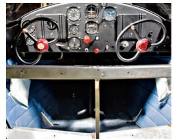
Unlike most airplanes, in which pedals control the rudders, the Ercoupe used **hand controls** to maneuver the rudders, ailerons (hinged sections on wings) and a steer-able nose.
