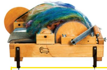
Davidson uses a **drum carder** to combine bits of silk and mohair with roving to create multi-textured yarn. She feeds various fibers under the small drum, which mesh with fibers on the larger drum as she turns the crank.
