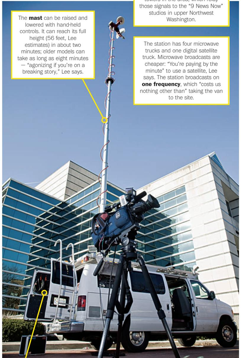
The **mast** can be raised and lowered with hand-held controls. It can reach its full height (56 feet, Lee estimates) in about two minutes; older models can take as long as eight minutes — "agonizing if you're on a breaking story," Lee says.
