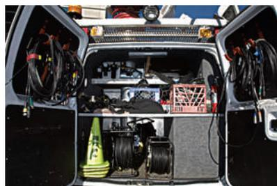
The back of the van contains about **800 feet of cable**, used for microphones and video cameras that feed into the van, as well as power cables.
