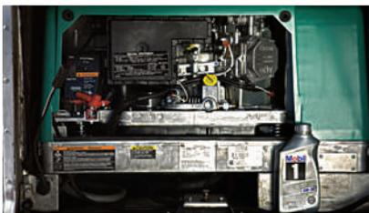
A seven-kilowatt gas **generator** powers the truck's electric equipment. "Maintaining this generator is critical to us, because we lose the news operations of this truck if it fails," Lee says.
