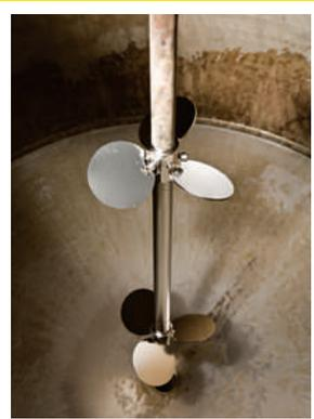
Whiskey production starts in the 1,200-liter stainless-steel mash tank. **Propellers** mix ground organic rye with boiling water for six hours. "This is essentially a big crock pot," Harris says.
